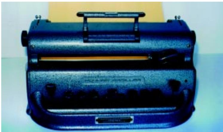
Fig. 13. Máquina Perkins Braille.
